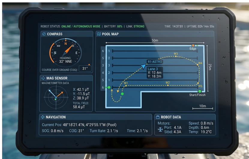
Figure 4.4: An HMI: from your computer, you can see the state of your DD-Boat and control it
