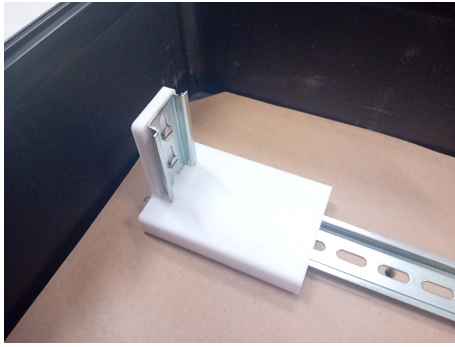
Figure 5: Support piece that was added
