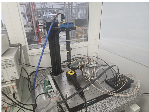
(a) Experimental setup: static suspension with microscope view over the electrodes.
