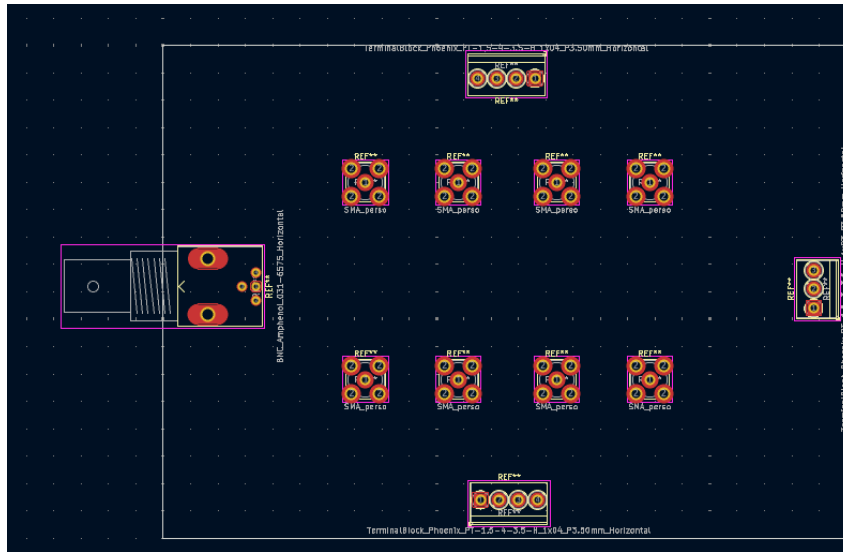
Figure 3.3: PCB layout with SMA connectors and footprints for multipliers and amplifiers.
