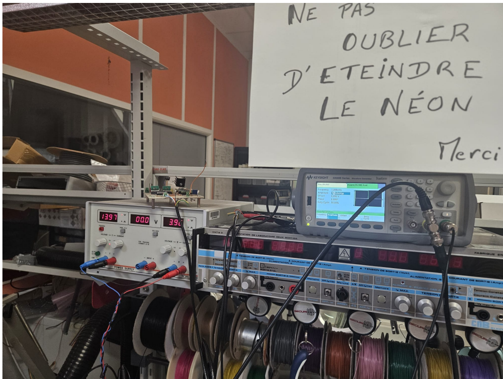
Figure 3.6: Signal source used for generating the rectangular (DC reference) and sinusoidal inputs.
