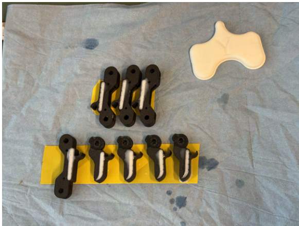
Figure 6.4: Moulding of the fingers using resin
