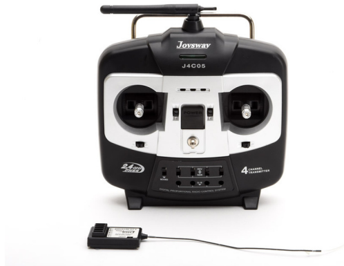
Figure 8: The Joyway J4C05 Remote controller and its J5C01R receiver
