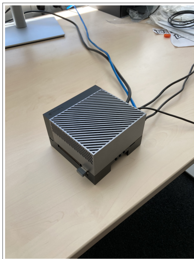
Figure 3: NVIDIA Jetson AGX Orin development board serving as the main computing platform.
