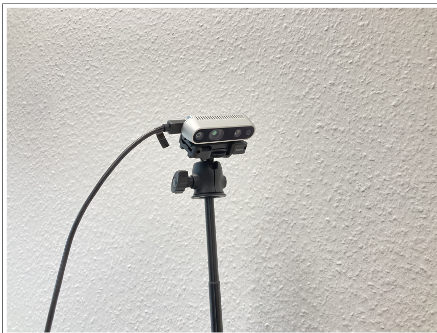
Figure 2: Intel RealSense D435i camera mounted for optimal workspace coverage.
