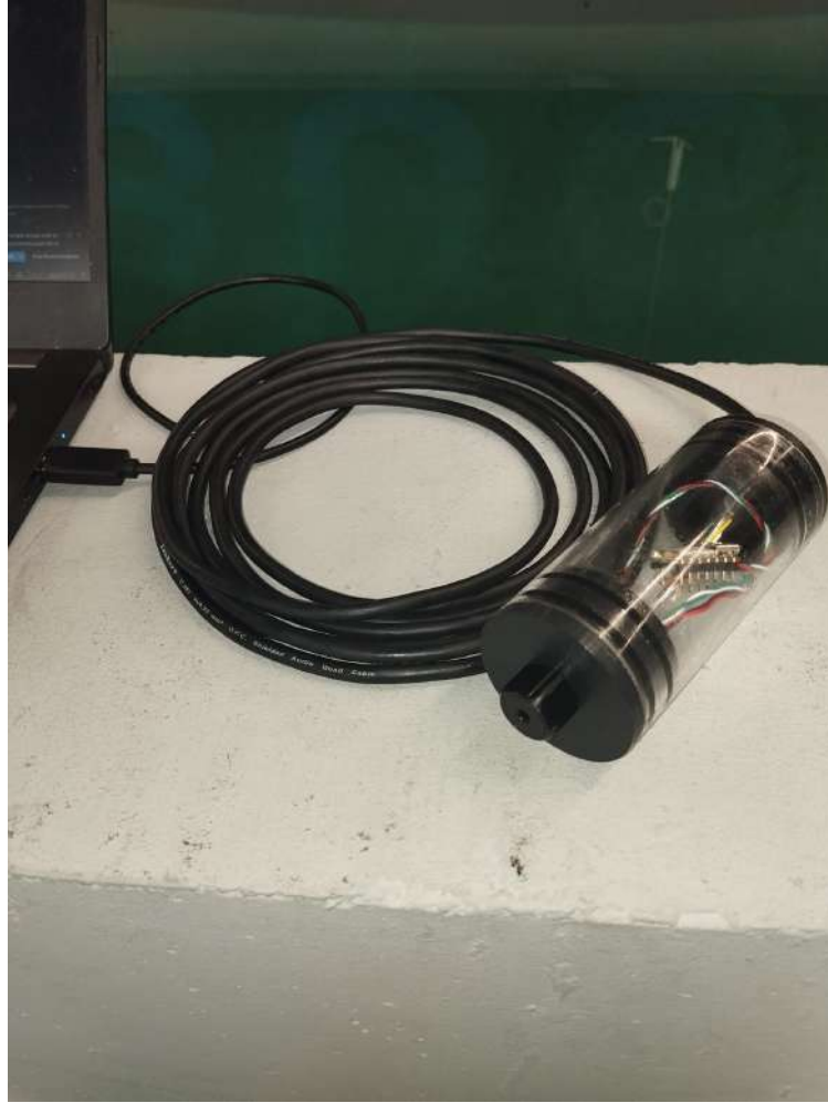
Figure 3.2: BAR30 measurement setup used for static and dynamic characterization campaign.
