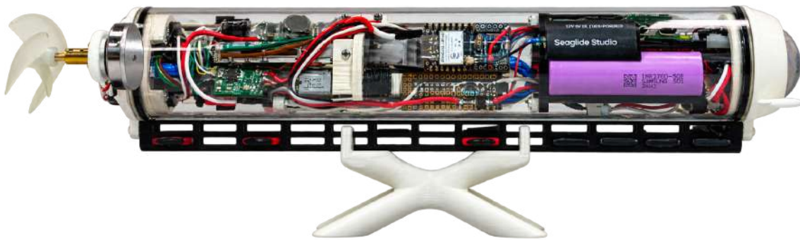
Figure 3.3: V2 prototype: more compact integration and reorganized electronics.
