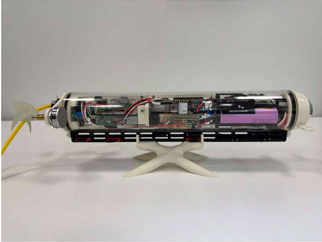
Figure 1.1: Side view of the final prototype, with acrylic tube, internal integration, and external support frame.
