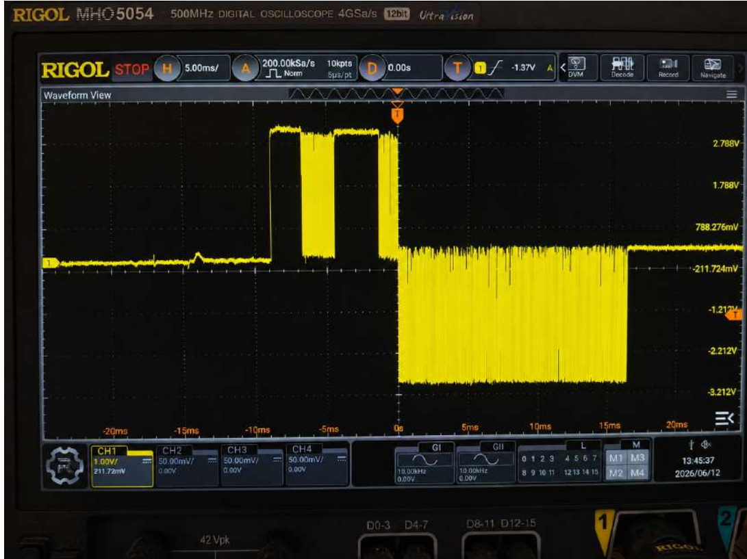
Figure A.6: Oscilloscope capture showing a transient/noise event during control-chain initialization.
