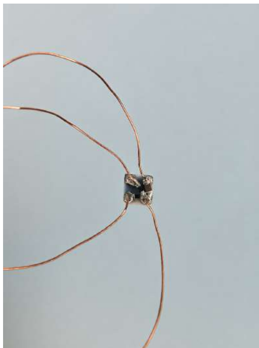
Figure A.5: MS5837-30BA pressure sensor micro-soldering before encapsulation.
