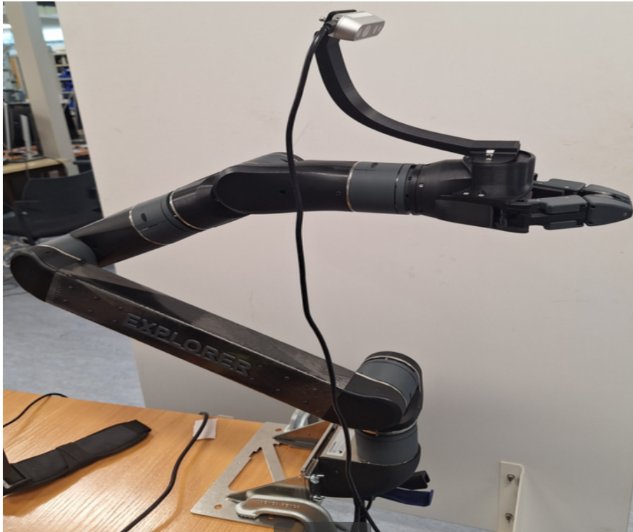
Figure 3.2: Orthopus Explorer robotic manipulator used during the experiments
