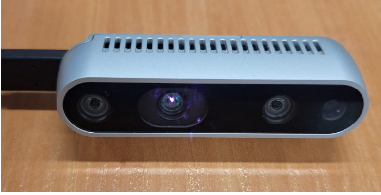
Figure 3.3: Intel RealSense D435 RGB-D camera used for visual perception
