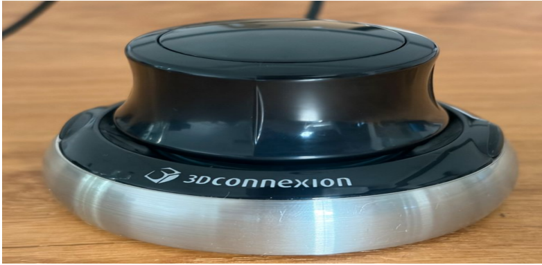
Figure 3.4: 3Dconnexion SpaceNavigator joystick used for user supervision
