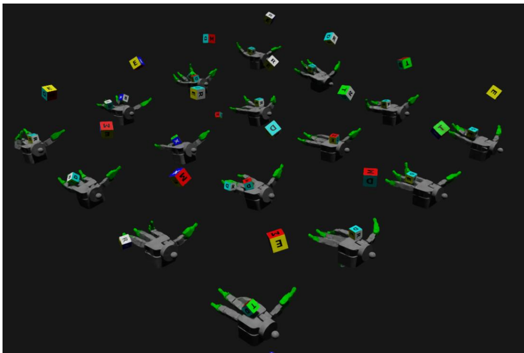
Figure 4: Allegro Hand V4 parallelized environment in Isaac Sim.
