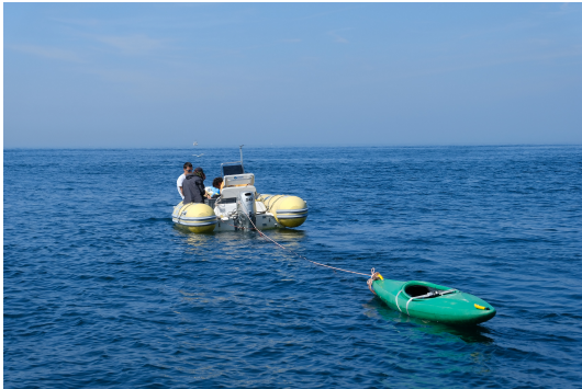
Boatbot towing a magnetometer
